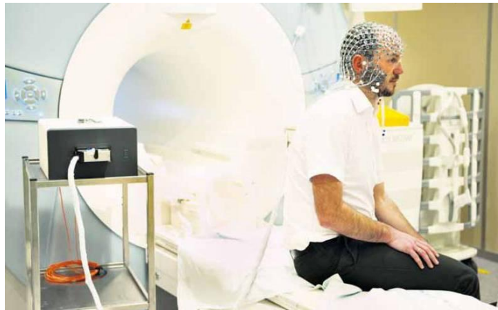
fMRI with 256 MR-compatible EEG channels
